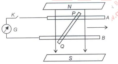
(a) Suppose K is open the rod is moved with a speed of 12 cm s<sup>-1</sup> in the direction shown in the figure. Give the polarity and magnitude of the induced emf.
