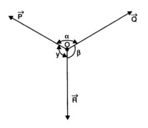
If three forces  $\vec{P}, \vec{Q}$  and  $\vec{R}$  are acting on a particle O in directions given by angles  $\alpha$ ,  $\beta$  and  $\gamma$ , then, the particle O is in equilibrium, when
