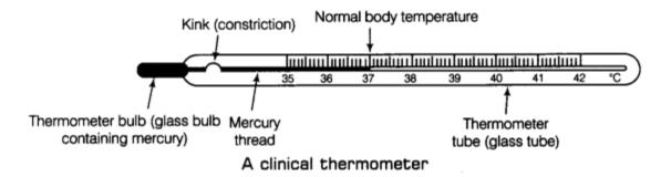
Just above the bulb containing mercury, a clinical thermometer has a kink in its glass tube which is to prevent the back flow of mercury into the thermometer bulb when the thermometer bulb is removed from the mouth of a patient. This kink prevents the mercury level in the thermometer tube from falling on its own. Due to this, we can read the correct body temperature of the patient even after removing the thermometer bulb from his mouth.
