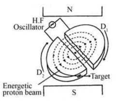
**Construction:** The construction of a simple cyclotron is shown in figure above. It consists of two-semi-cylindrical boxes  $D_1$  and  $D_2$ , which are called dees. They are enclosed in an evacuated chamber. The chamber is kept between the poles of a powerful magnet so that uniform magnetic field acts perpendicular to the plane of the dees. An alternating voltage is applied in the gap between the two dees by the help of a high frequency oscillator. The electric field is zero inside the dees
