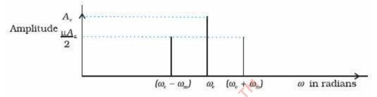
Modulation index:- It is defined as the ratio of amplitude of modulating signal to the amplitude of carrier wave. Mathematically it can be written as
