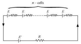
Equivalent *emf* of *n* cells connected in series is given as:
