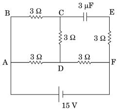
In the circuit shown in the figure, find the total resistance of the circuit and the current in the arm CD.
