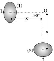
Two very small identical circular loops, (1) and (2), carrying equal currents I are placed vertically (with respect to the plane of the paper) with their geometrical axes perpendicular to each other as shown in the figure. Find the magnitude and direction of the net magnetic field produced at the point O.
