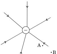
Figure shows the field lines due to a negative point charge. Give the sign of the potential energy difference of a small negative charge between the points A and B.
