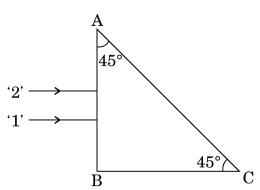
**QB365 - Question Bank Software**Two monochromatic rays of light are incident normally on the face AB of an isosceles right-angled prism ABC. The refractive indices of the glass prism for the two rays '1' and '2' are respectively 1.3 and 1.5. Trace the path of these rays after entering through the prism.
