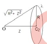
The field at an axial point of a circular loop of radius R and linear charge density  $\lambda$ , is given by
