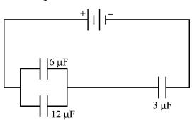
In the following arrangement of capacitors, the energy stored in the 6  $\mu F$  capacitor is E. Find the value of the following :
