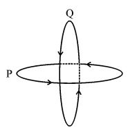
Two identical coils P and Q each of radius R are lying in perpendicular planes such that they have a common centre. Find the magnitude and direction of the magnetic field at the common centre of the two coils, if they carry currents equal to I and  $\sqrt{3}$  I respectively.
