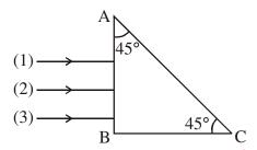
Three rays (1, 2, 3) of different colours fall normally on one of the sides of an isosceles right angled prism as shown. The refractive index of prism for these rays is 1.39, 1.47 and 1.52 respectively. Find which of these rays get internally reflected and which get only refracted from AC. Trace the paths of rays. Justify your answer with the help of necessary calculations.
