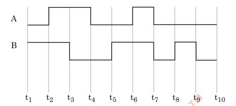
Two signals A and B are used as inputs of a NOR gate. Draw the output wave form.
