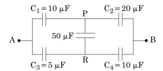
Calculate the equivalent capacitance between points A and B in the circuit below. If a battery of 10 V is connected across A and B, calculate the charge drawn from the battery by the circuit.
