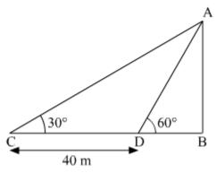
Let AB is the tower and BD is the length of the shadow when sun's altitude is  $60^{\circ\circ}$ . Let, AB be *x* m and BD be *y* m.
