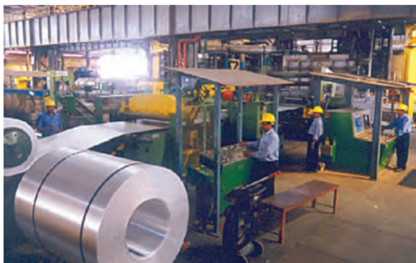
Fig. 6.6: Strip casting mill at smelter of NALCO
