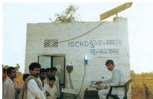
Fig. 5.11: Solar operated electronic milk testing equipment
