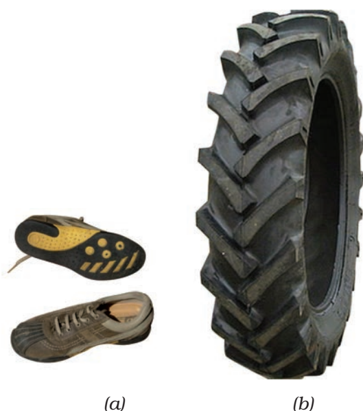
Fig. 12.11 : (a) Soles of shoes and (b) tyres are treaded to increase friction
