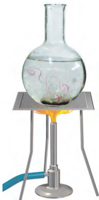
Fig. 4.9 Convection of heat in water
