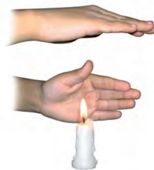
Fig. 4.10 Transfer of heat by convection in air
