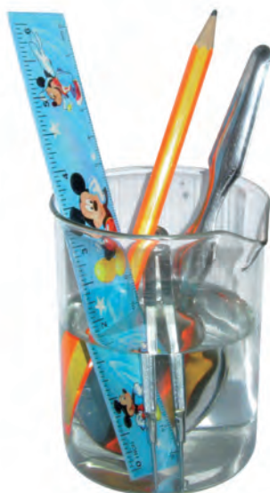
Fig. 4.8 Conduction of heat by different materials
