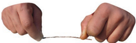
Fig.3.4 Splitting the yarn into thin strands
