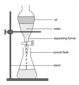
Separation of 2 immiscible liquids is done using a separating funnel. The above figure shows a separating funnel clamped to a stand. In this case the mixture to be separated contains oil and water.
