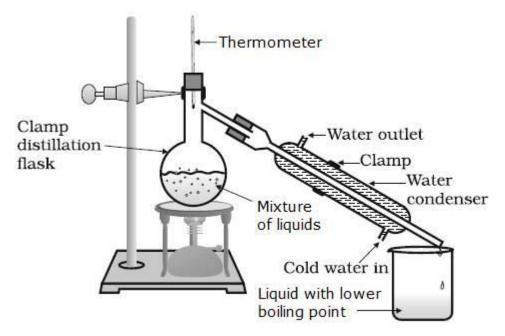
The mixture of liquids is taken in a round bottom flask and is heated. The liquid component with a lower boiling point starts to escape from the mixture and the gas is passed through a condenser. The cold water helps to condense the gas into its liquid form and is collected in a beaker.
