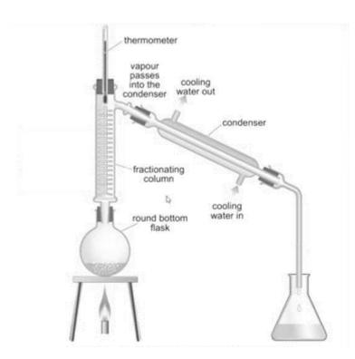
Fractional distillation is the process used to separate a mixture of miscible liquids whose boiling points differ by less than 25°C. The experimental setup is similar to that of distillation except for a fractionating column which is filled with glass beads.
