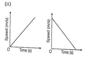
The first graph represents a body which is moving with a uniform acceleration and the second graph represents a body which is moving with uniform retardation.
