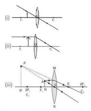
The image is virtual, erect and larger than the object.
