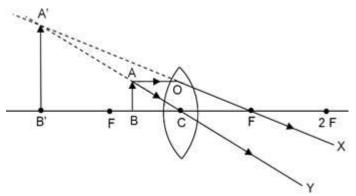
Real image of various sizes can be obtained when the object is placed beyond the principal focus.
