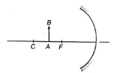
**Answer:** The mirror is the concave mirror and the object is kept between Centre of curvature and focus.
