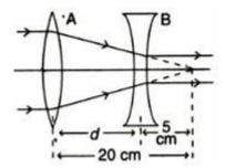
As the incident ray is parallel to the principal axis. Therefore in absence of concave lens it will form an image at focus of convex lens.
