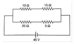
Answer: Here, the resistances  $10\Omega$  and  $15\Omega$  are connected in series and also the resistances  $20\Omega$  and  $5\Omega$  are also connected in series.
