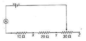
**Answer:** The current when it is connected to x is 0.6 A, so net resistance is 10 ohms so the cell voltage is  $10 \times 0.6 = 6$  V.
