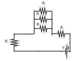
Q. 5. In the circuit shown below, calculate the net resistance of the circuit.
