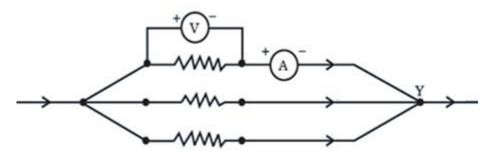
• We will close the switch and note the readings. Similarly, we will switch the position of voltmeter to resistances  $R_2$  and  $R_3$  and observe the readings.
