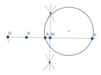
Step5: Take distance MB in compass keep the needle on point M and draw a semicircle as shown
