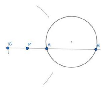
Step4: Keeping the distance in the compass same as that of in step3 keep the needle on B and mark arcs intersecting the arcs drawn in step3. Join these intersection points we get the perpendicular bisector of CB at M
