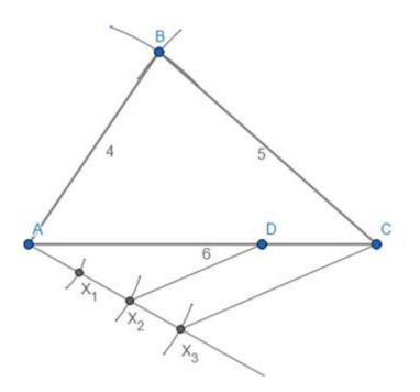
Step7: construct line parallel to BC from point D and mark the intersection point with AB as E thus  $\Delta ADE \sim \Delta ACB$  is ready
