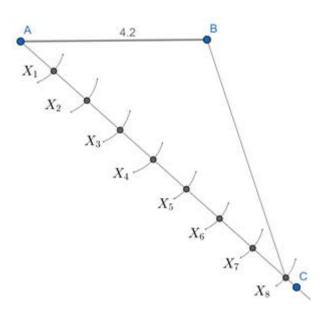
Now we have to divide the segment AB in ratio 5:3, i.e. 5 parts and 3 parts.
