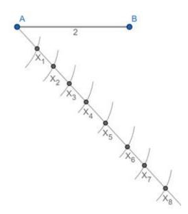
Step4: Join X<sub>5</sub>B. Extend AB and draw a line parallel to X<sub>5</sub>B which intersects the extended AB at C. Hence C divides externally the segment AB
