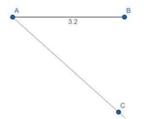
Step3: take any distance in compass and keep the needle of the compass on point A and draw an arc intersecting the line AC. Name the intersection point as  $X_1$ . Keeping the distance same in compass keep the needle on point  $X_1$  and mark an arc intersecting AC at  $X_2$ . Draw 8 (3:5 given ratio 3 + 5 = 8) such parts i.e. upto  $X_8$
