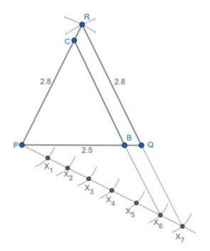
Now to construct the circumcircle of  $\Delta$ PBC. The centre of circumcircle is the intersection of perpendicular bisectors, and the radius is the distance from the centre to any vertex of the triangle. We will draw perpendicular bisector of PC and BC
