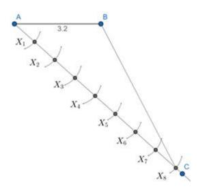
Now we have to divide the segment AB in ratio 3:5, i.e. 3 parts and 5 parts.
