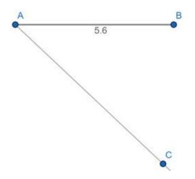
Step3: take any distance in compass and keep the needle of the compass on point A and draw an arc intersecting the line AC. Name the intersection point as  $X_1$ . Keeping the distance same in compass keep the needle on point  $X_1$  and mark an arc intersecting AC at  $X_2$ . Draw 13 (5:8 given ratio 5 + 8 = 13) such parts i.e. upto X<sub>13</sub>
