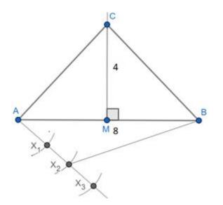
Step7: Now extend AB and draw a line parallel to  $X_2B$  from  $X_3$  intersecting AB at D
