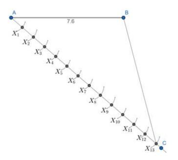
Now we have to divide the segment AB in ratio 5:8, i.e. 5 parts and 8 parts.
