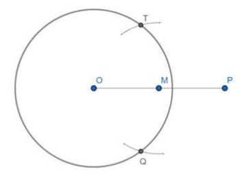
Step5: Draw lines passing through PT and PQ which are the required tangents and measure length PT and PQ them with scale
