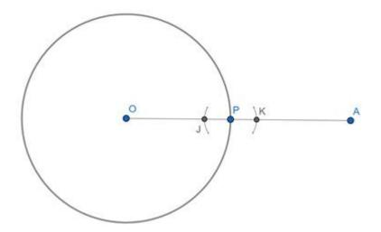
Step4: Take any distance in compass greater than JP, keep the needle on point J and mark arcs above and below OA.
