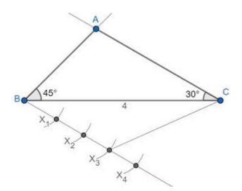
Step6: Now extend BC and draw a line parallel to  $X_3C$  from  $X_4$  intersecting BC at D
