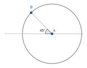
Step3: Using protractor draw a line perpendicular to AB from point B because the radius is perpendicular to the tangent. Mark the intersection of this line with a line passing through the centre as C hence CB is the required tangent at  $45^{\circ}$
