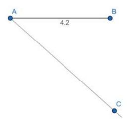
Step3: take any distance in compass and keep the needle of the compass on point A and draw an arc intersecting the line AC. Name the intersection point as  $X_1$ . Keeping the distance same in compass keep the needle on point  $X_1$  and mark an arc intersecting AC at  $X_2$ . Draw 8 (5:3 given ratio 5 + 3 = 8) such parts i.e. upto  $X_8$
