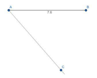
Step3: Take any distance in compass and keep the needle of the compass on point A and draw an arc intersecting the line AC. Name the intersection point as  $X_1$ . Keeping the distance same in compass keep the needle on point  $X_1$  and mark an arc intersecting AC at  $X_2$ . Draw 13 (5:8 given ratio 5 + 8 = 13) such parts i.e. upto  $X_{13}$
