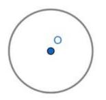
Step2: Now take 6 cm in compass keep the needle on point 0 and draw a circle. This is the outer circle. Take any point P on the outer circle
