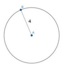
Step2: Using protractor draw the line at  $45^{\circ}$  to AB from point A and mark its intersection point with a circle as C join AC
