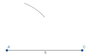
Step3: take distance 5 cm in compass keep the needle of the compass on point C and mark an arc intersecting the arc drawn in step2. Mark intersection point as B join AB and AC
