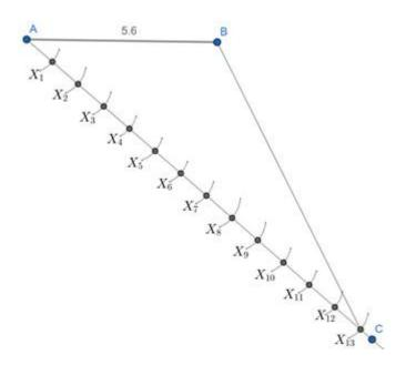
Now we have to divide the segment AB in ratio 5:8, i.e. 5 parts and 8 parts.
