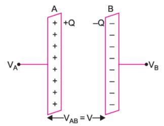
**Ans. (a)** When a capacitor is charged by a battery, work is done by the charging battery at the expense of its chemical energy. This work is stored in the capacitor in the form of electrostatic potential energy.
