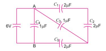
Ans. The equivalent capacitance of C1 and C2 in series
