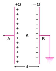
Let A be the area of each plate, 'd' the separation between the plates, K the dielectric constant of medium between the plates. If  $\sigma$  is the magnitude of charge density of plates, then
