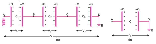
In series' first plate of each capacitor has charge +Q and second plate of each capacitor has charge –Q i.e., charge on each capacitor is Q.
