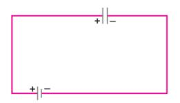
**Ans. (i)** In the steady state no current flows through capacitor because, we have two sources (battery and fully charged capacitor) of equal potential connected in opposition.
