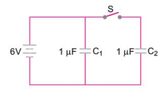
Ans. When switch S is closed, p.d. across each capacitor is 6V
