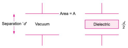
Capacitance with dielectric of thickness 't'
