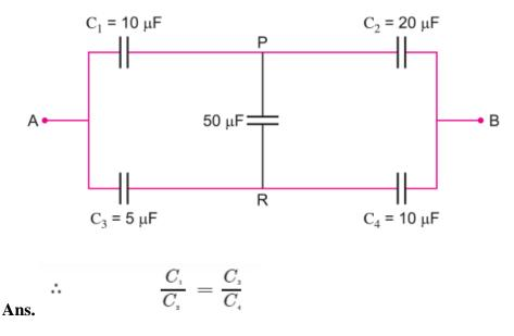
This is the condition of balance so there will be no current across PR (50  $\mu$ F capacitor) Now C<sub>1</sub> and C<sub>2</sub> are in series
