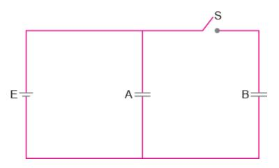
**Ans.** Two capacitors are connected in parallel. Hence, the potential on each of them remains the same. So, the charge on each capacitor is
