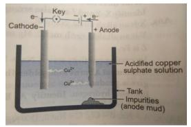
insoluble impurities settle down at the bottom of the anode and are known as anode mud.
