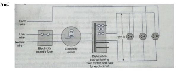
A fuse in a circuit prevents damage to the appliances and the circuit due to overloading. Otherwise, the appliances or the circuit may be damaged.
