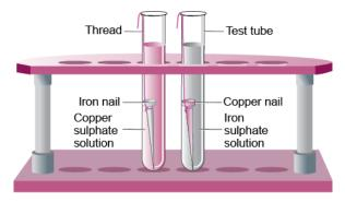
You will observe that the reaction has occurred in the test tube containing iron nail and copper sulphate solution. Iron takes the sulphate away from copper. You see that a reaction takes place and copper is left by itself. Now, we can say that iron has displaced copper from copper sulphate.
