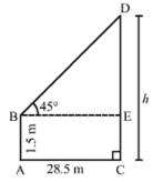
Draw  $BE \perp CD$ , let CD = h meters. Then,  $AB = 1.5 m, BE = AC = 28.5 m and \ \angle EBD = 45^{\circ}$  DE = (CD - EC) = (CD - AB) = (h - 1.5)m. In right  $\triangle BED$ , we have:
